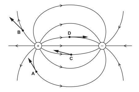
**32** Lightning can occur between a charged cloud and the Earth's surface when the electric field strength in the intervening atmosphere reaches 25 kN C<sup>-1</sup>. The diagram shows the electric field between the base of a cloud and the Earth's surface.
