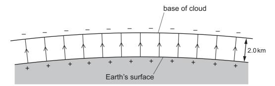
What is the minimum potential difference between the Earth and the base of a cloud, 2.0 km high, for lightning to occur?
