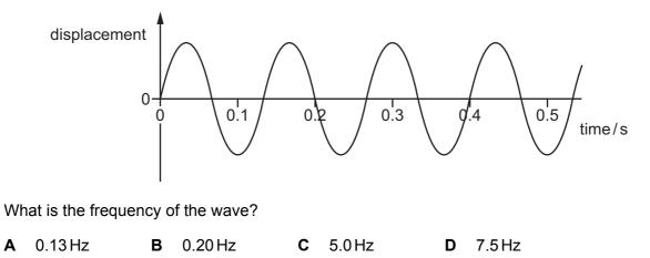
24 An electrical signal is displayed on a cathode-ray oscilloscope (c.r.o.).
